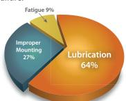
Sixty-four percent of bearing failures are lubrication related. Less than 9% of bearings reach their L10 design life expectancy.
